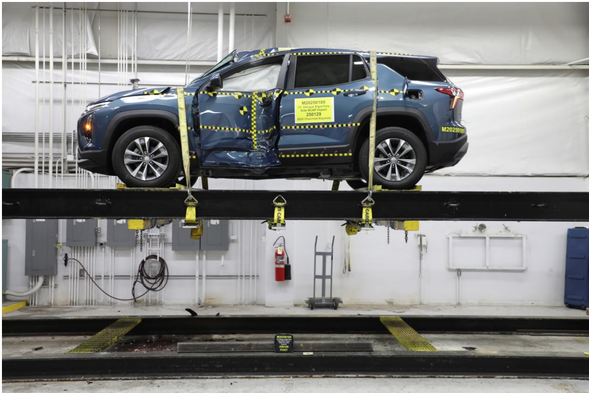
No. 065 FMVSS No. 301 Static Rollover 0 Degrees
