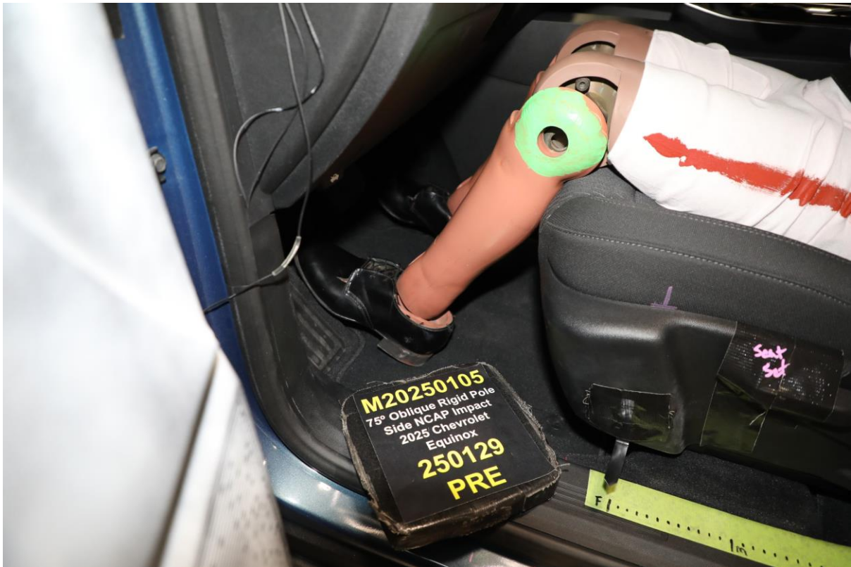
No. 032 Pre-Test Placement of Dummy Feet
