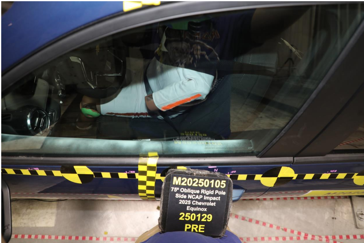
No. 040 Pre-Test Dummy and Door Clearance View
