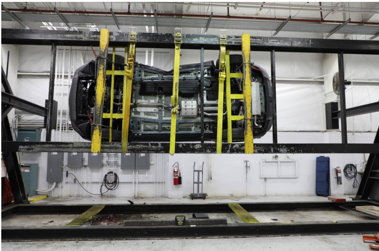
No. 068 FMVSS No. 301 Static Rollover 270 Degrees
