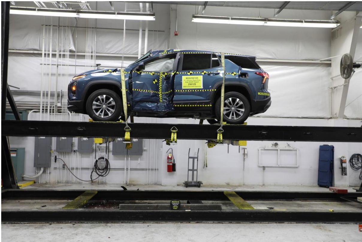
No. 069 FMVSS No. 301 Static Rollover 360 Degrees
