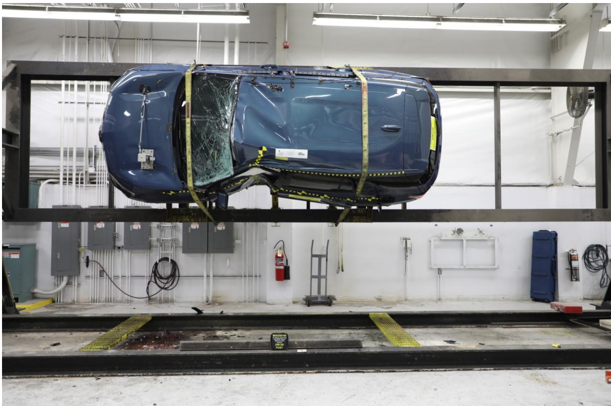
No. 066 FMVSS No. 301 Static Rollover 90 Degrees
